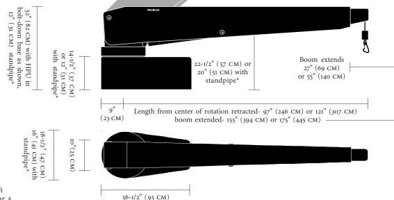
\*Subtract 3" (18 CM) from the lift height figures above when using a standpipe vs. the bolt-down base illustrated here.
