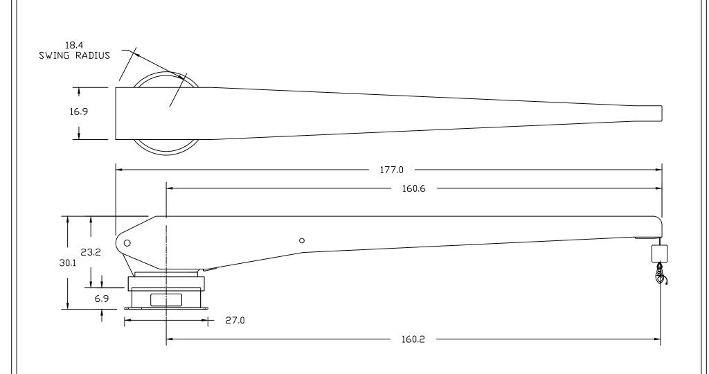
RATED FOR 2500LBS STANDARD BOOM LENGTHS FROM 136-180 STD CABLE TRAVEL=26 FT MAX BOOM ELEVATION ANGLE=67° MIN REACH FOR 160 BOOM SHOWN=51″ @ 67° NORMAL ROTATION=348.5 DEGREES
